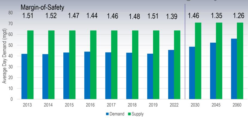
With reactivation of the Housatonic Wellfield the Greater Bridgeport System has adequate supply to meet increased demands and make all required reservoir releases.
