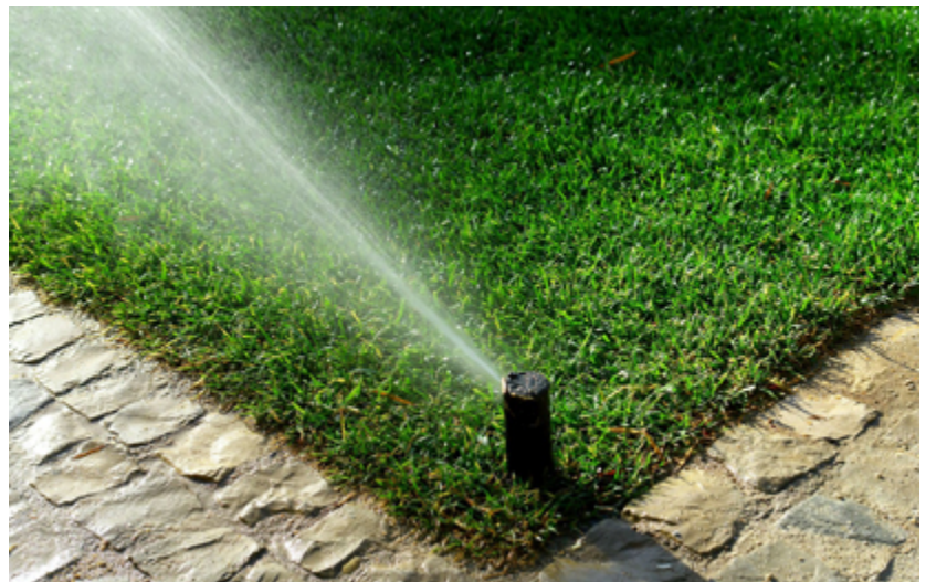
Ensure that irrigation heads are directed at turfgrass, not sidewalks or other impervious surfaces. Photo courtesy of http://www.hrriirrigation.com
